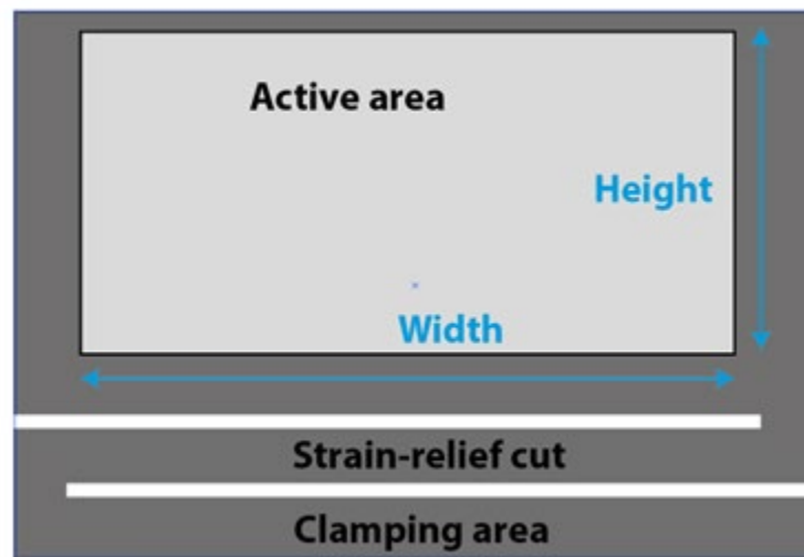
Figure 1 Schematic layout of the silicon crystal. The thin active membrane (5 mm width, >3 mm height) is mechanically isolated from the clamping area by a laser-defined strain-relief cut, ensuring stress-free operation.
