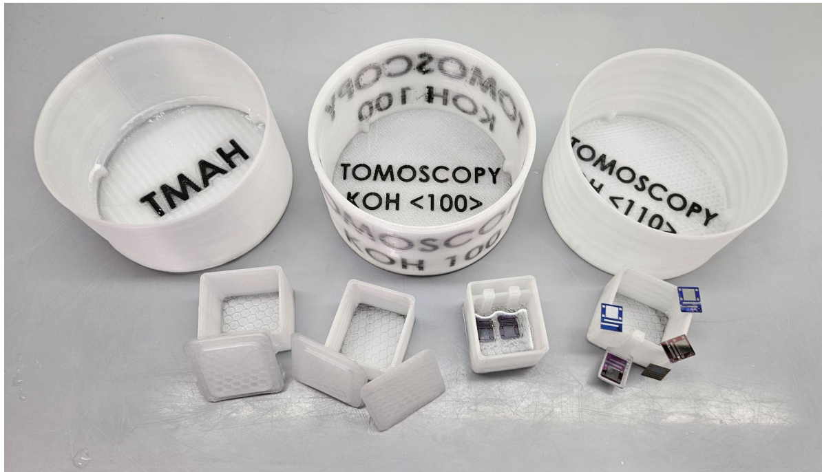
Figure 8 – Photo of some of custom-designed polypropylene containers and holders developed for the safe handling and chemical processing of fragile silicon membranes. All components were 3D printed in-house and optimized for compatibility with KOH and TMAH solutions, enabling stress-free wafer manipulation during long-duration etching cycles.
